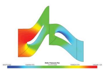
Fig. 9. Static Pressure at middle cut of the blade
