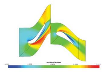
Fig. 8. Relative Mach number at middle cut of the blade
