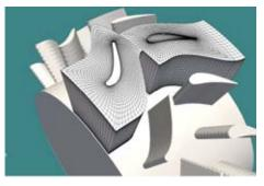
Fig. 6. Turbine geometry with O-Grid
