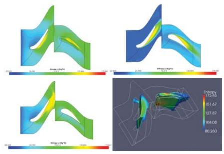
Fig. 7. 2D and 3D contours plots of Entropy (left upper corner - shroud, right upper corner - middle, left lower corner - shroud, right lower corner - 3D contours of largest entropy)
